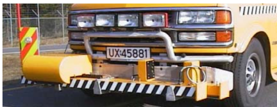
Figure 4 – Front mounted hosting beam for multiple measurement systems; mean profile depth, evenness and transverse profile.
