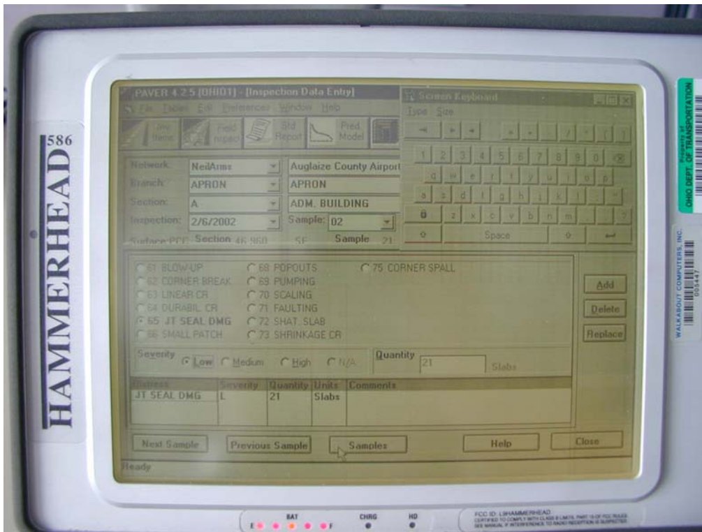
Figure 5: Pen computer set up for field data entry. Keypad is used to enter data.
