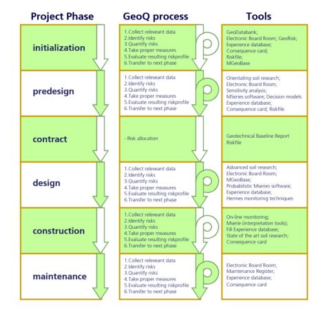
In the next chapter you can see an example of GeoQ in practice. Here is shown that risk management of earthworks pays out. For the Betuweroute, the Sliedrecht-Gorinchem section, built on a very soft soil underground, active risk management in the design and construction stage led to an optimised design and a building time within the requirements for lower costs than estimated originally.
