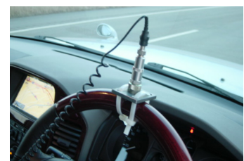
Photo 2 The pickup of a vibration meter fixed to the steering wheel
