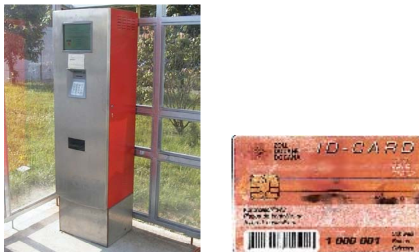
Figure 6 – Self-service machine and ID-card for users non equipped with OBU
