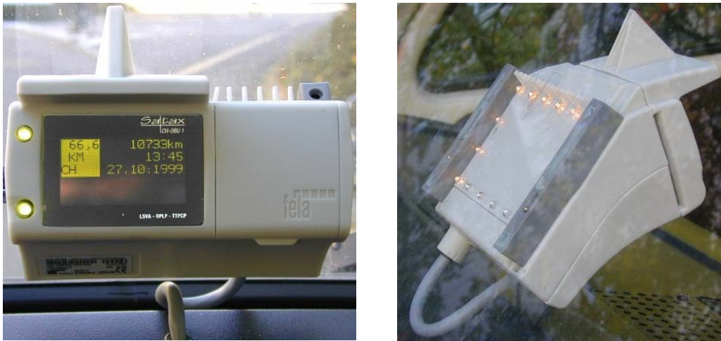
Figure 3 - LSVA On-Board Unit (OBU) front and rear side
