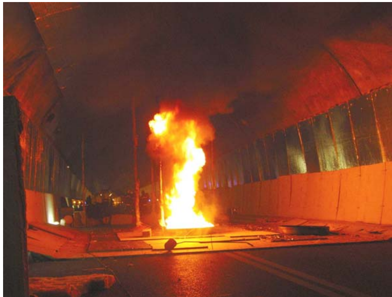
Figure 2 – View of a 1.4 MW fire, at the end of the transient ventilation phase. The stratification and the longitudinal confinement of the smoke are controlled
