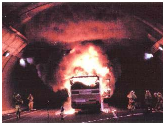
Figure 7. Tunnel fire test of large-scale tunnel
