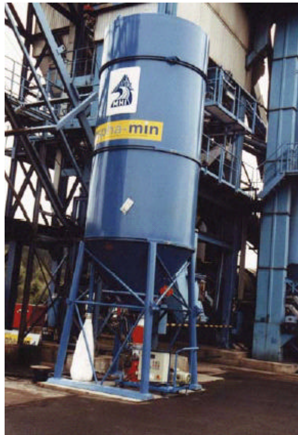
Figure 2 Adding the aspha-min®
