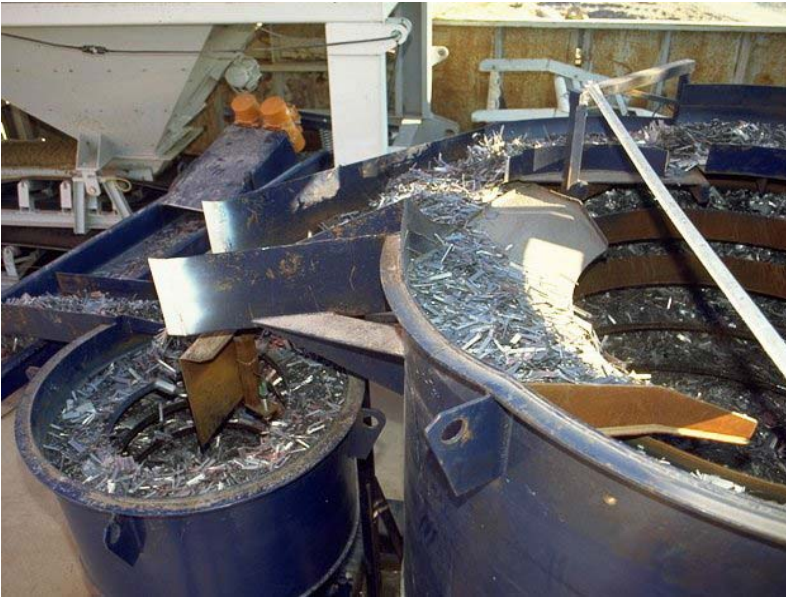
Figure 2 – Fiber dosing system using Bekaert Dramix 80/60 in continuous plant
