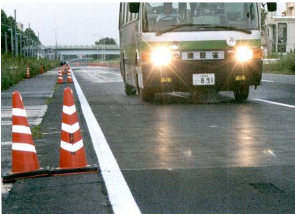
Figure 7 - Apparatus for wet skid resistance
