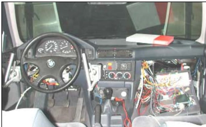
Figure 12: The central control unit and bus clamps for preparing the input and output clamps are located in the glove compartment.
