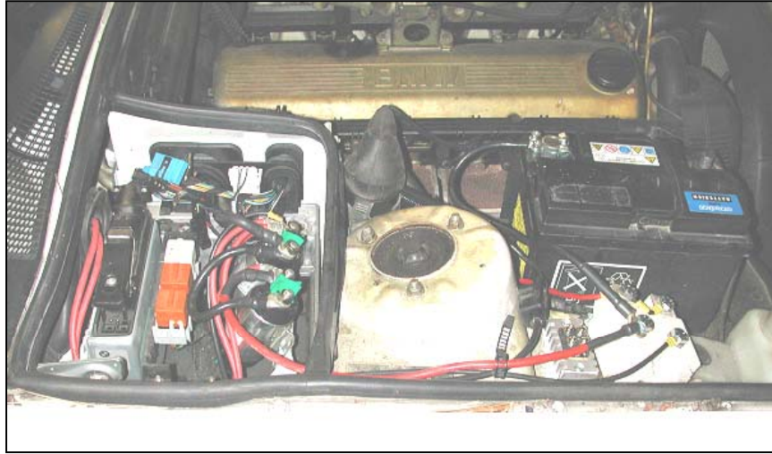
Figure 11: The power relays (up to 1,000 amps) for switching the batteries are visible on the left, while the power diodes for separating the batteries are shown on the right.
