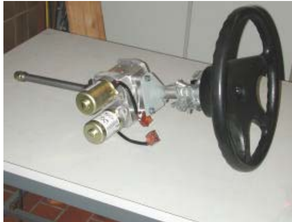
Figure 5: Steering column with the two steering motors and fully functional steering wheel
