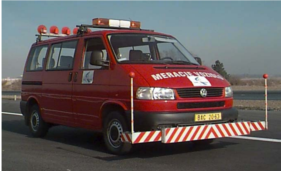
Picture 3 The diagnostic device PROFIOLOGRAPH GE
