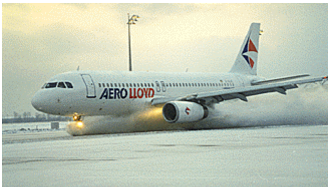
Figure 2 - Example of test carried out under Joint Winter Runway Friction Measurement Programme
